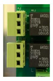
Warning Shock Hazard. Caution 230V mains voltage could be present at these relays that may require isolation elsewhere.
