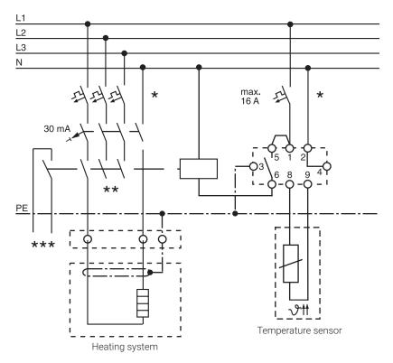
Two- or four-pole electrical protection by circuit-breaker may be needed for local circumstances, standards and regulations \* Depending on the application, one- or three-pole circuit-breakers or contactors may be used \*\* Optional: Potential-free circuit-breaker for connection to the BMS \*
