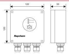
A Green LED Heating cable on B Red LED Sensor break C Red LED Sensor short-circuit
