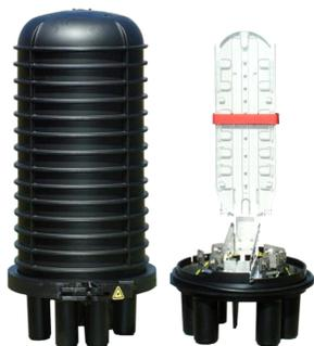
FOSC™400 A4 Fiber Optic Splice Closure, Heat Shrink Cable sealing, one pre-installed 24-splice tray, ground feedthrough lugs, with test valve
